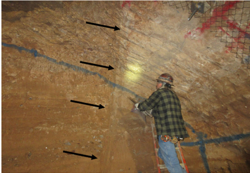
Arrows pointing to the fault plane, showing evidence of historic seismic activity of the faults present within PULSE.
